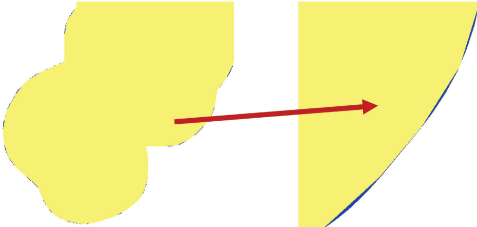
Figure 2. Visual assessment of the differences occurring while generating buffer zones in ArcGIS (blue) and QGIS (yellow)
