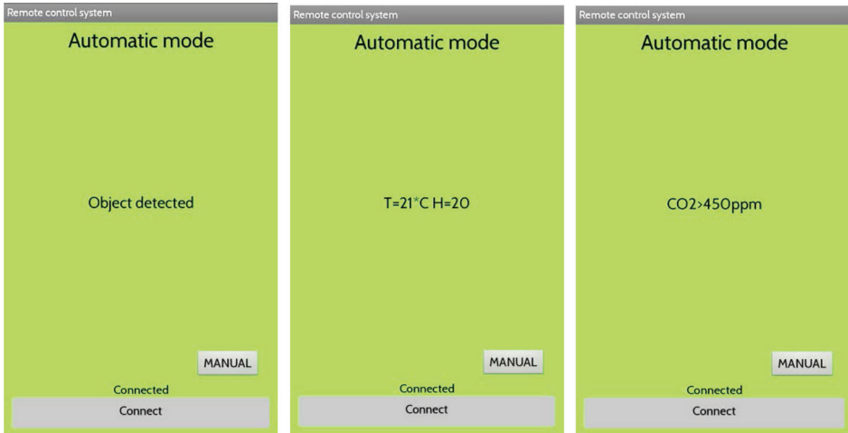
Figure 9. Data displayed by the mobile application in automatic mode
