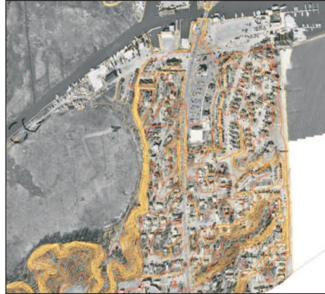
Fig. 53. Orthophotograph with horizontal lines (a sample)
