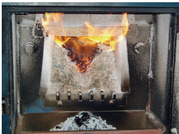
Figure 5. Detailed view into the burner at the end of pure sorrel combustion
