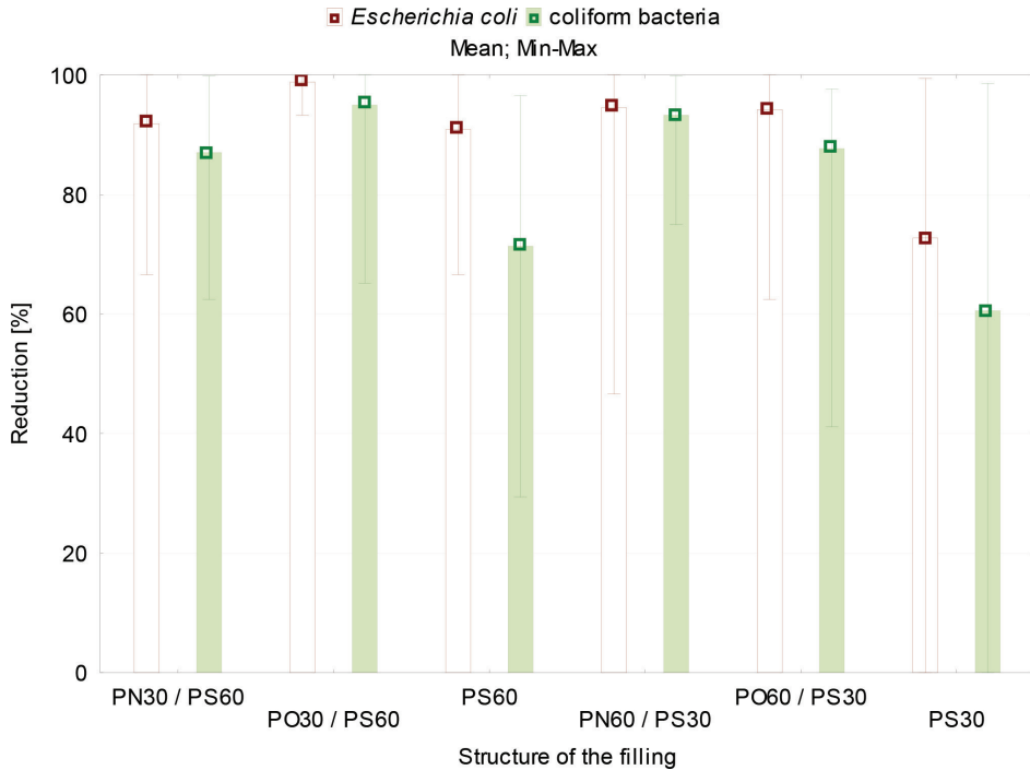
Figure 4. Box-plot chart for the reduction of Escherichia coli and coliforms in treated wastewater in filtration beds of the various structure of the filling
