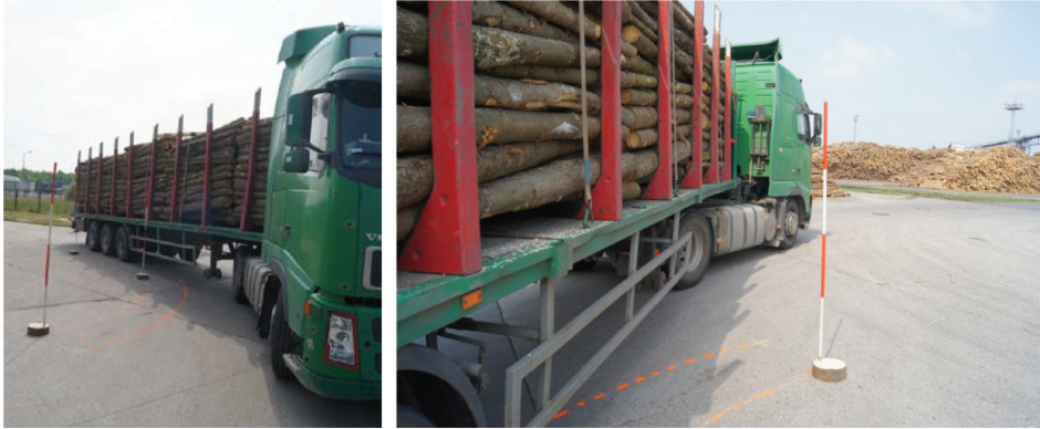
Figure 3. Testing the trajectory for a combination composed of a truck and a semi-trailer
