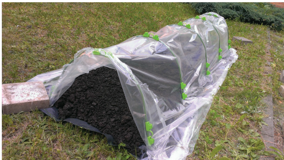
Figure 1. The tunnel for sludge drying on the semi-technical scale
