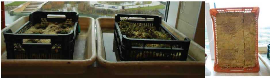
Figure 3. Set up of experiment: a) tray 1: mineral wool waste + extensive green roof substrate + Lysimachia punctata ; b) tray 2: mineral wool waste + extensive green roof substrate + Jovibarba sobolifera ; c) tray 3: mineral wool waste (reference site).
