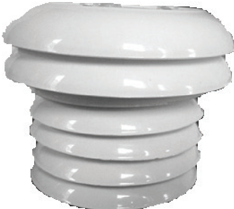
Figure 3. Radiation shield in which the sensor was placed
