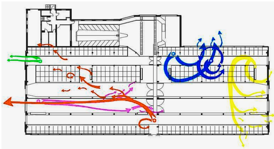
Figure 3. The movement of smoke from smoke generators in six characteristic points of the main hall with curtain walls wide open – an overview
