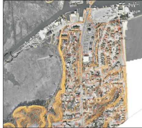
Fig. 53. Orthophotograph with horizontal lines (a sample)
