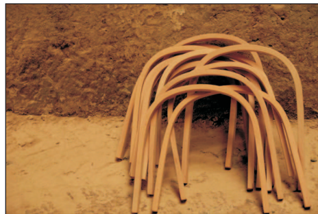
Phot. 97. Bending beech wood in hot steam
