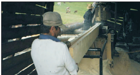
Phot. 120. Sawing of logs with a circular saw [Boğan 2005]
