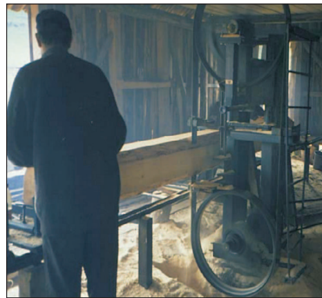
Phot. 121. Sawing of logs with a vertical band saw [Boğan 2005]
