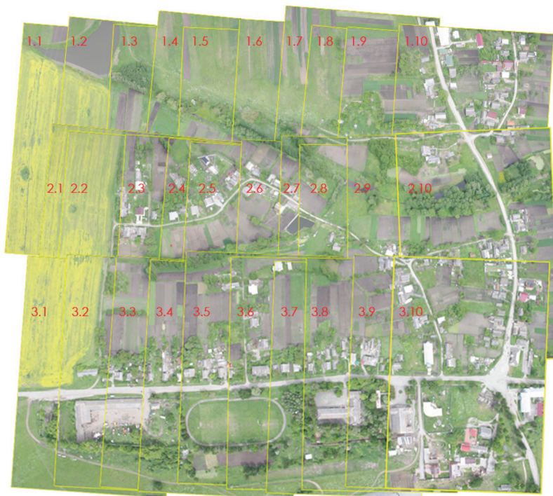
Figure 10. Aerial image mosaicking which combine three routes. The height of imagery is 300 m. The imagery is made by a digital camera Canon EOS 450 D (three routes, 10 photos each).
